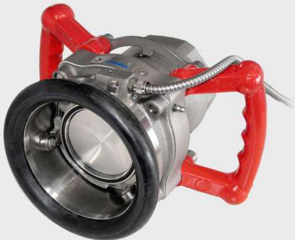
Hose unit with magnetic switch The switch indicates if the hose unit is fully connected to a standard tank unit. Can be used to start pumps, activation of brakes on road tankers, etc.
