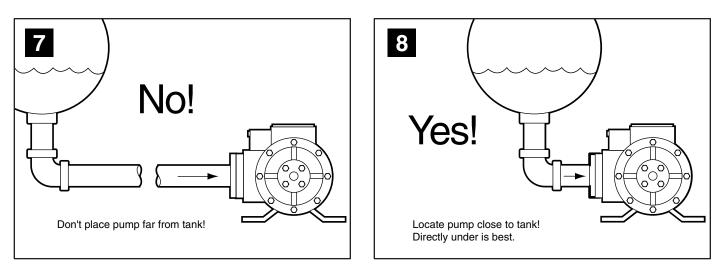
It is best to allow the pump to be fed by gravity flow to give stable, trouble-free operation.
