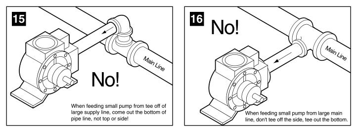
Low capacity flow through large lines often does not sweep out vapor. Flow occurs like liquid in a flume. Drawings 15 and 16 would allow vapor slugs to be drawn into the small pump causing erratic performance. Drawing 17 shows the best chance for stable feed into a small pump from a large line.
