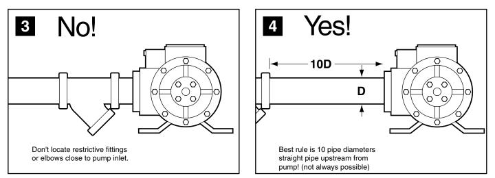
Turbulence caused by flow interference close to the pump accentuates incipient cavitation.
