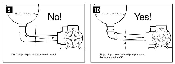
Vaporization in the pump inlet line can displace liquid in the pump so that pump may start up in a dry condition. A slope toward the pump of only an inch or two in a 10 foot run will allow vapor to gravitate back into the tank and be replaced with liquid.
