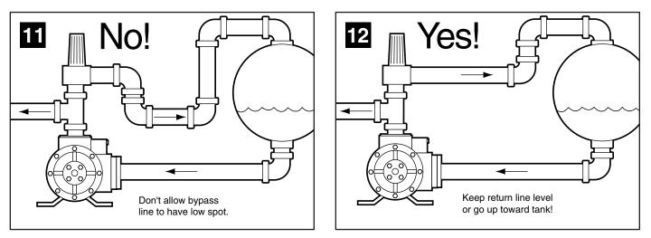
Low spots in bypass line can collect liquid which prevents normal vapor passage for priming purposes just like the P trap in the drain of a kitchen sink. This is not a problem for bypass lines where vapor elimination is not required.
