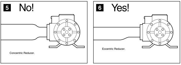
An eccentric reducer should always be used when reducing into any pump inlet where vapor might be encountered in the pumpage. The flat upper portion of the reducer prevents an accumulation of vapor that could interfere with pumping action.
