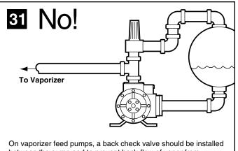
between the pump and to prevent back-flow of vapor from entering pump.
